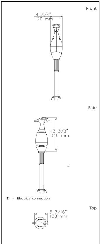
Electric Supply voltage: 110-120 V/1 ph/50/60 Hz **Total Watts:** 0.35 kW Plug type: USA NEMA 5-15P Key Information: External dimensions, Width: 5 7/16" (138 mm) External dimensions, 4 3/4" (120 mm) Depth: External dimensions, 30 1/8" (765 mm) Height: **Shipping width:** 11 7/16" (290 mm) Shipping depth: 27 3/16" (690 mm) Shipping height: 7 1/16" (180 mm) **Shipping weight:** 12 lbs (5.3 kg)
